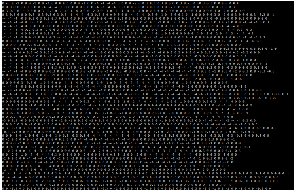
Fig. 1: The principle of the program: 0, 0.3 – neutral centers; 0.8 - positive center; -1, -2 – cells in the process of oxidation; -4 - dead cells; -3 - cluster center
