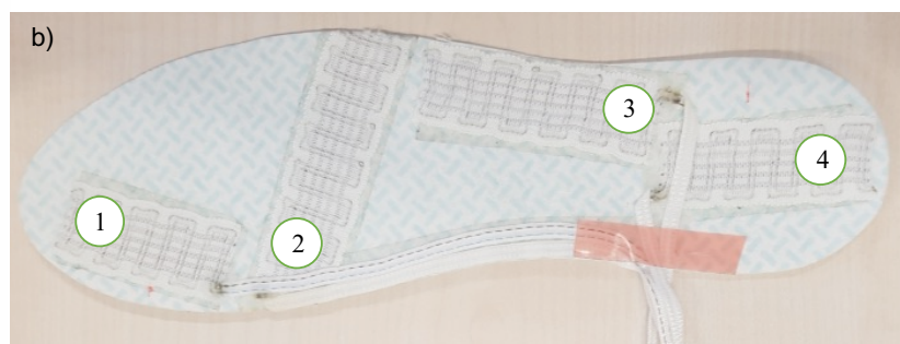
Fig. 1: a) The effect of melt volume flow rate on the electrical conductivity of PA6/MWCNT-CB nanocomposite fibres, b) Sensing example for a pressure sensor fiber for smart textiles.
