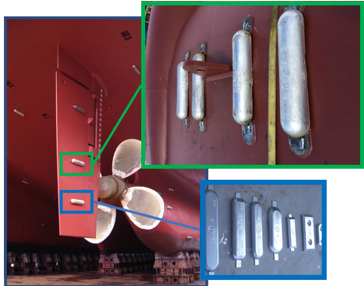
Fig.2: Types and positioning example of SACP anodes [2] – [4].
