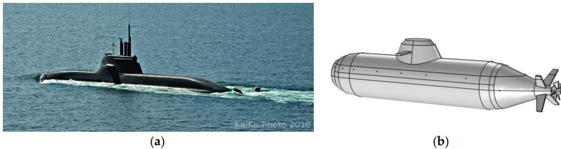
Figure 1. (a) Photo of a type 212A submarine and (b) the geometry of the numerical submarine model for simulating the AEP signature.
