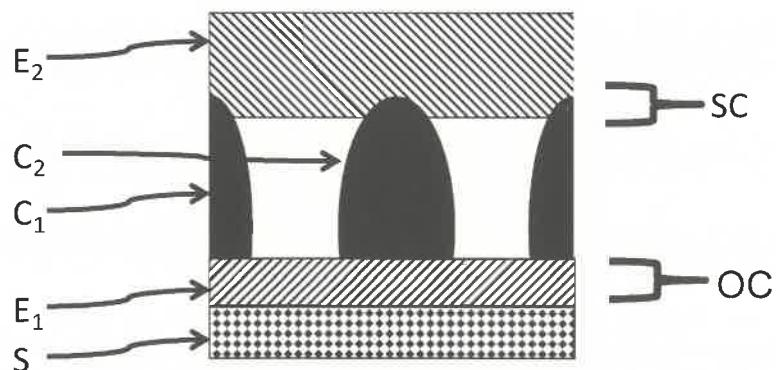
step of applying a second electrode, so that the tip of the mu-cone is joined to the second electrode.
