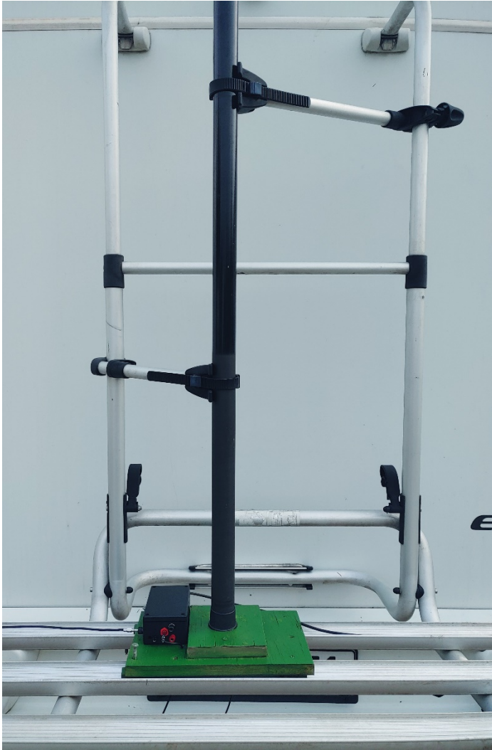
Figure 2: Set up of the vertical radiator mast on the bicycle rack. The match box is at the bottom left next to the mast.
