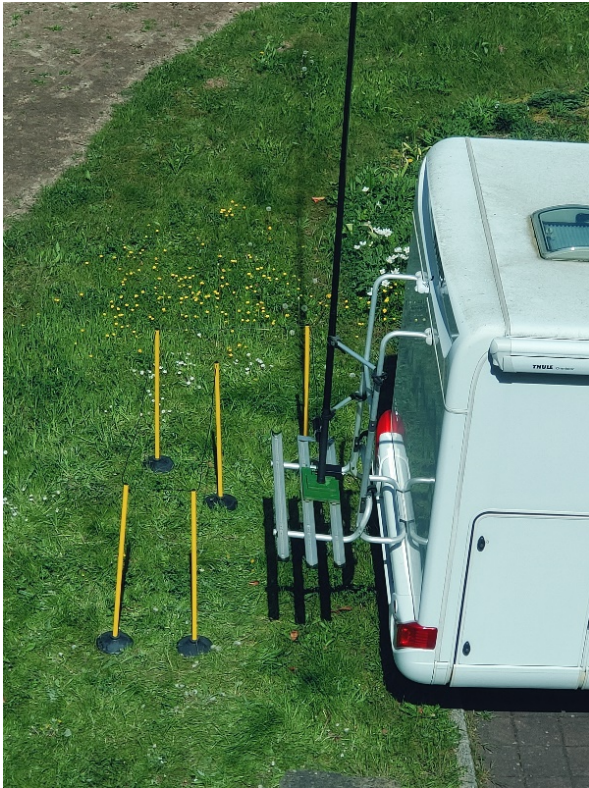
Figure 1: Vertical antenna placed on the motor home's bicycle rack
