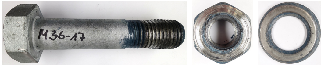
Figure 38 M36 HV - Microgleit HV-paste LP440 test specimen after tightening
