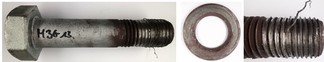
Figure 35 M36 HV - Molykote 1000 spray test specimen after tightening
