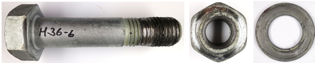
Figure 32 M36 HV - Gleitmo WSP 5040 test specimen after tightening
