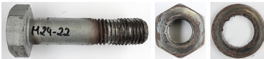
Figure 23 M24 HV - Molykote 1000 spray test specimen after tightening
