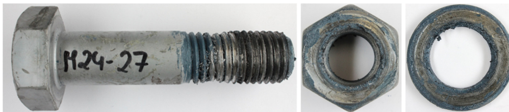
Figure 26 M24 HV - Microgleit HV-paste LP440 test specimen after tightening
