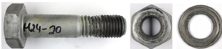
Figure 20 M24 HV - Gleitmo WSP 5040 test specimen after tightening
