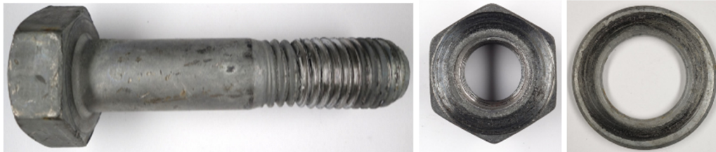
Figure 17 M24 HV - Factory provided test specimen after tightening
