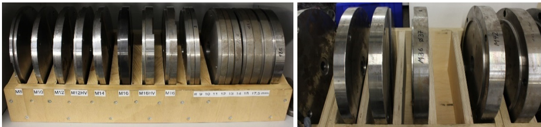
Figure 11 Different shims with minor diameter (left) and major diameter (right) at IML laboratory of University of Duisburg-Essen
