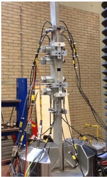
Instrumented slip factor specimen in test rig. Slip was measured at both PE and CBG positions
